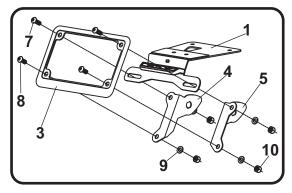
Route license plate light and turn signal wires through the hole in (No. 1) 12122-FEBKT, fender eliminator bracket and through the lower rear cowl. Secure (No. 1) 12122-FEBKT, fender eliminator bracket to subframe using the four stock fender bolts and (No. 9,10) 6MMWASHER, 6MMLN, washer and nut as shown.
