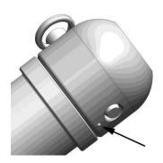
3) Install the plastic top 45-1099 using the removable pin 45-5099. Important: One side of the puck has a small hole drilled beneath the main hole. Install the pin so that the end of the pin with the ball is on the same
