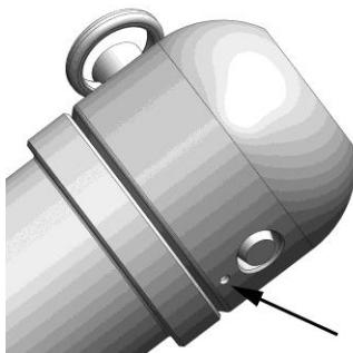
3) Install the plastic top 45-1099 using the removable pin 45-5099.
