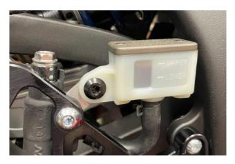
6) Secure the rear brake reservoir to the bracket using the included hardware. From the outside in, the order or parts is the 6x20mm bolt, 6mm washer, reservoir, 12-3240 bracket and then the 6mm locknut. Adjust the bracket angle as needed.
