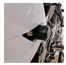
3) Torque the left side bolt before removing the right side OEM bolt
