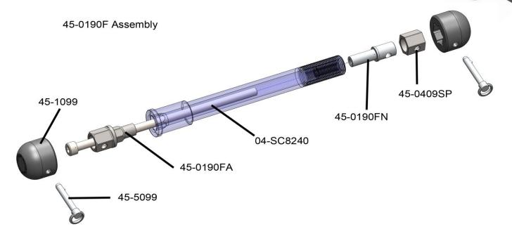
A note for racers: If your tech inspector wants you to safety wire these (most will not) then you need to orient the pins so that the safety wire acts to pull the pin into the puck.
