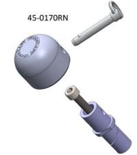
5) Install the plastic top using the removable pin. **Important:** One side of the puck has a small hole drilled beneath the main hole. Install the pin so that the end of the pin with the ball is on the same side as this small hole. The OEM nut will slide right over the base. In order to remove the rear wheel, you will only need to remove the puck on this side of the rear axle.
