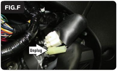
10 Unplug the crank position sensor connector (Fig. F).
