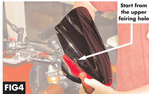
Fig 4. Installing the ZG windscreen, place and align the screen to the holes on top of the fairing. Start off by inserting the ZG fasteners (provided) on the 2 top fairing holes as shown above. Complete the install with the 2 remaining fasteners at the bottom.
