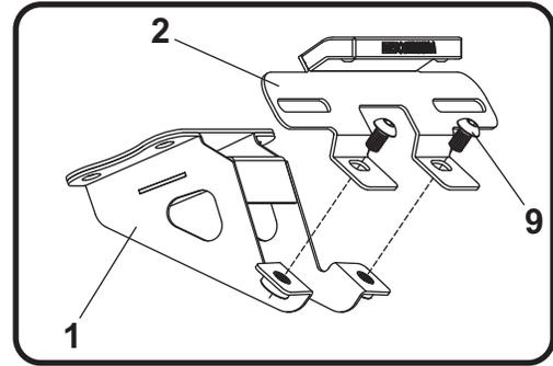
3. Install (No. 1) *13700-FEBKT*, fender eliminator bracket to subframe using the stock bolts.
