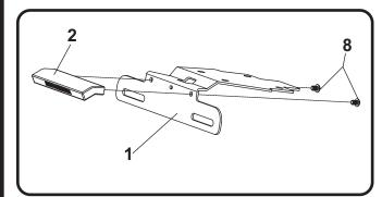
2. Install (No. 1) 11100-FEBKT, fender eliminator bracket using (No. 7) M6X14BHS, 6mm button head screws. Route wires through hole in the bracket and beneath the passenger seat.
