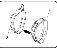
3. Install (No. 5) 27-61*M*, exhaust clamp over (No. 1) *11600-435-1*, tailpipe. Do not torque at this time.
