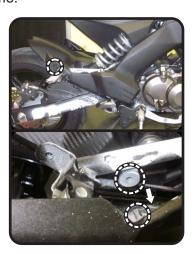
6. Remove the right side footpeg plate bolt closest to the rider footpeg. Bolt will be replaced in a later step.
