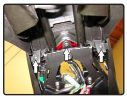
6. Remove the stock fender assembly by removing the bolts securing fender assembly in place.
