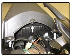
Remove the five screws securing the tail light assembly and remove tail light by carefully pulling toward the rear of the vehicle.
