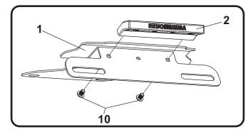
Install (No. 1) 12300-FEBKT, Yoshimura fender eliminator bracket to subframe using the stock bolts. See diagram below for correct hole mounting location depending on model.
