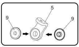
5. Install (No. 4) *HT SHLDR77*, muffler clamp heat insulator onto (No. 3) *MCYM5-GCBX(-X)*, muffler clamp.
