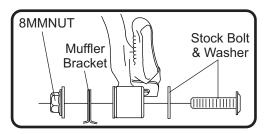
8. Torque muffler mount bolt to factory specification.
