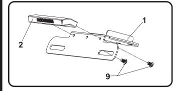
Note: Route license plate light wire through the hole under the fender eliminator bracket.
