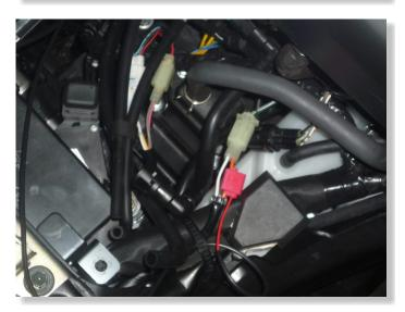
CONNECT X-TRE RED WIRE TO DRANGE WIRE OF REAR BRAKE LIGHT SWITCH CONNECTOR. (TRANSPARENT, 2-POLE CONNECTOR
