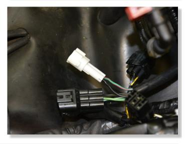
INSERT THE BLACK AND GREEN/RED WIRES INTO THE LARGER WHITE, 2-POLE CONNECTOR.
