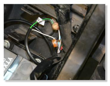
CONNECT THE X-TRE BLACK/WHITE WIRE TO BROWN/RED WIRE END, WHICH IS AT THE WIRING HARNESS SIDE.
