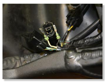
RELEASE AND REMOVE TWO TERMINALS FROM SMALLER, 6-POLE CONNECTOR. (WHITE/YELLOW AND BLACK WIRES)
