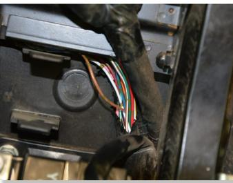
LOCATE ECU WIRING HARNESS UNDER MAIN SEAT, UNDER THE STARTER RELAY. LOCATE THE BROWN/RED WIRE AMOUNG THE ECU WIRES. CUT THE BROWN/RED WIRE.
