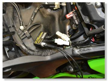
PLUG X-TRE CONNECTORS IN-LINE WITH THE WHITE, 2-POLE CONNECTORS.
