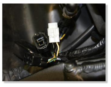
INSERT THE BLACK AND WHITE/YELLOW WIRES INTO THE SMALLER WHITE, 2-POLE CONNECTOR.
