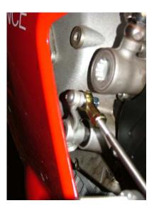
**For GP Shift** – Flip the gear change actuator (attached to the shift shaft on the motor) approximately 180-degrees from the OEM position. Adjust the actuator on the spline until it makes as close to a 90-degree angle with the shift rod as possible.
