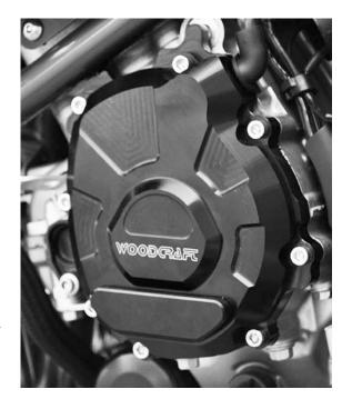
3) Attach the stator, pickup and wire retainer using the OEM hardware to the Woodcraft cover. Be sure that the retainer does not contact the rotor before assembly. **IMPORTANT - USE**
