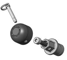
2) Put a 19mm box end wrench on the hex of the assembly and tighten the 8mm allen bolt to lock the assembly in place.
