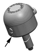
3) Install the plastic top using the removable pin. **Important:** One side of the puck has a small hole drilled beneath the main hole. Install the pin so that the end of the pin with the ball is on the same side as this small hole. The pin should be installed so that the ring is on the top half of the slider.
