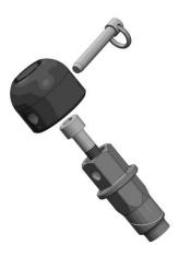
2) Tighten the 8mm allen bolt to lock the assembly in place. You should hold the base with a wrench while doing this to ensure you can fully lock the axle side in place.
