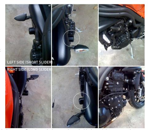
or 8 mm countersunk bolt provided. The bolt passes first through the non threaded hole and then screws into the threaded hole on the far side of the base. The plastic is undersized on the far side of the slider to act as a locknut for the bolt
