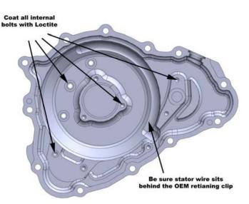
**MOUNTING BOLTS.** Be sure to use a newer bottle and coat the threads completely and allow the threadlocking compound to fully set before use.
