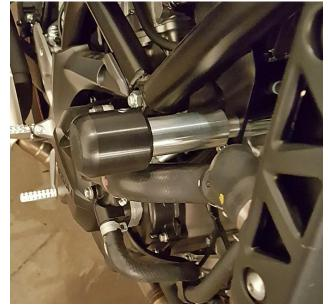
3) Slide the plastic slider over the top of the base and secure it in place using the 8mm countersunk bolt provided. The bolt passes first through the non threaded hole on the aluminum base and then screws into the threaded hole on the far side. The plastic is undersized on the far side of the slider to act as a locknut for the bolt.
