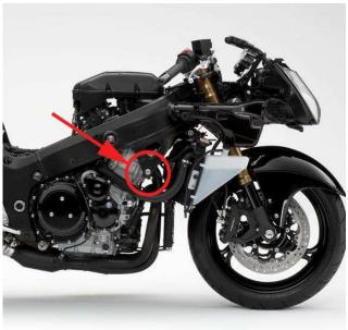
3) This kit requires the cutting of the bodywork on both sides. With the bases in place, attempt to trace the outline of the base on the inside of the bodywork in order to find the center of the hole to drill for the puck. Look through the hole to ensure that it is in the center of the frame slider base.
