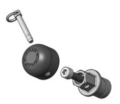
2) Put a 19mm box end wrench on the hex of the assembly and tighten the 8mm allen bolt to lock the assembly in place.
