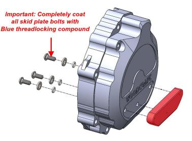
The generic cover at the right shows both o-rings and optional washers on the skid plate bolts. If your skid plate did not come with washers, simply put the o-ring directly beneath the head of the bolt.
