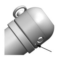
3) Install the plastic top using the removable pin. **Important:** One side of the puck has a small hole drilled beneath the main hole. Install the pin so that the end of the pin with the ball is
