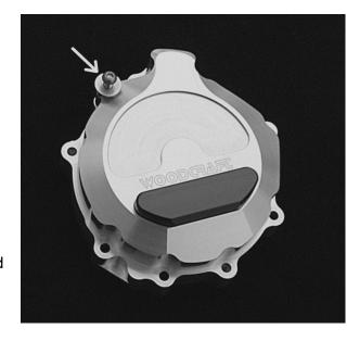
IMPORTANT - USE BLUE THREADLOCKING COMPOUND on the three skid plate mounting bolts. <u>Completely</u> coat the threads & allow time to cure before running!
