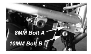
motor mount bolt and 8mm support bolt. Secure the slider puck base to the inner base using the supplied 10mm bolt. Coat with anti-sieze and torque all bolts to OEM recommended specifications (consult service manual).
