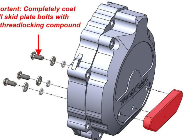
**IMPORTANT - USE BLUE THREADLOCKING COMPOUND on the three skid plate mounting bolts. Completely coat the threads & allow time to cure before running!**
