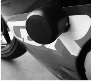
3) Slide the plastic slider over the top of the base and secure in place using the 8 mm countersunk bolt provided. The bolt passes first through the non threaded hole and then screws into the threaded hole on the far side of the base. The plastic is undersized on the far side of the slider to act as a locknut for the bolt
