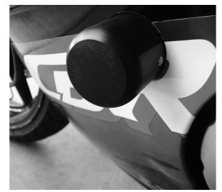
3) Slide the plastic slider over the top of the base and secure in place using the 8 mm countersunk bolt provided. The bolt passes first through the non threaded hole and then screws into the threaded hole on the far side of the base. The plastic is undersized on the far side of the slider to act as a locknut for the bolt
