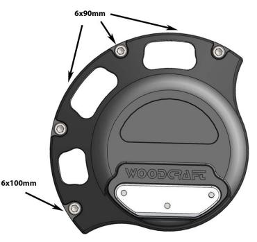
2) Install the Woodcraft cover using the included mounting hardware in the 4 locations shown above. Torque for these mounting bolts is about 7 ft-lbs.
