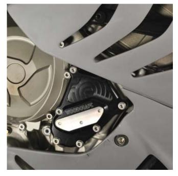
IMPORTANT - USE **BLUE LOCTITE** ON THE THREE SKID PLATE MOUNTING BOLTS. The bolts should be completely coated in Loctite and allowed to dry (see the directions on your Loctite bottle) before use.
