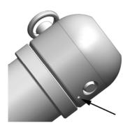
3) Install the plastic top using the removable pin.
