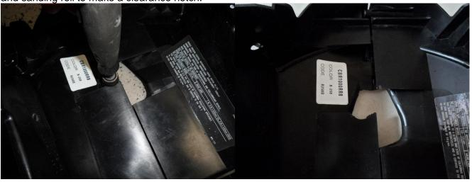
5. Using the base plate as a template mark were 6 X 30 bolts will go though. Remove base plate and use a 15/64 drill bit to drill holes.
