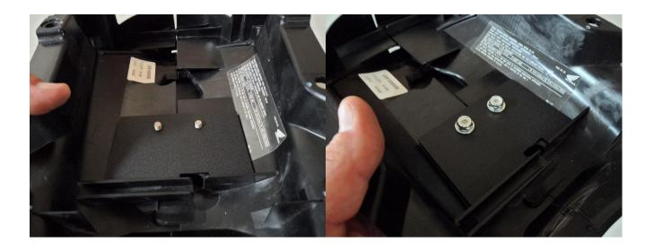
7. Reinstall fender. The seam of the bottom support plate should like up with the bodywork as it did before removal.
