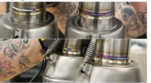
6. Install TBR muffler assembly to UTV in a sliding motion using the OEM rubber mounting points.
