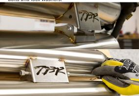
Install TBR slip tube. Use a thin layer of supplied antiseize on both slip fit joints. Attach with supplied hook springs.
