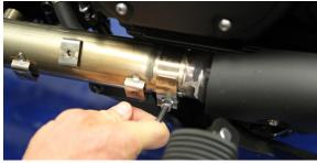
10. Reinstall O2 sensor to slip tube
