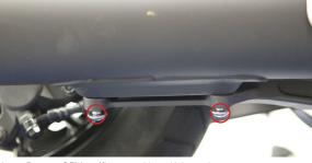
6. Remove OEM muffler assembly and joint gasket.
