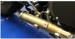
11. Install OEM heat shield onto TBR slip tube.
