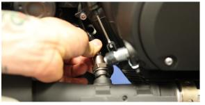
Remove lower muffler mounting bolts. These will be used with TBR bracket
