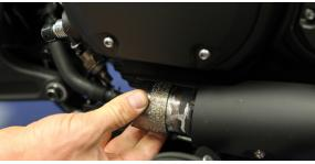
Remove OEM muffler bracket and bolts.
