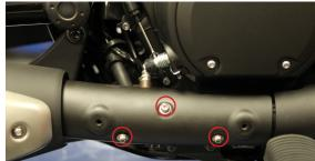
3. Loosen muffler barrel clamp.
