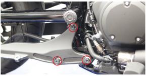
Install TBR muffler bracket using OEM bolts from lower muffler mount
