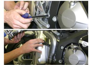
13. Loosen the OEM barrel clamp connecting the exhaust tube and header.
