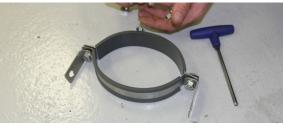
19. Attach muffler clamp assembly under the heat shield using the 2 OEM bolts and 6mm nuts.
