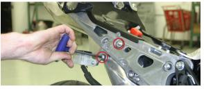
12. Remove right side driver's footpeg bolts and carefully remove the exhaust tube heat shield.
