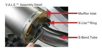
Attach the X-Lite<sup>™</sup> V.A.L.E.<sup>™</sup> assembly to the muffler canister using the 4 (four) 6mm x 14mm socket head cap screws. Leave loose for now.
