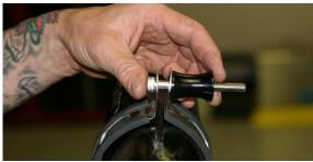
12. Install supplied O2 adapter. Install O2 sensor into O2 adaptor.
