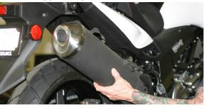
8. Install TBR mid-pipe using OEM mounting hardware and supplied 57mm barrel clamps.
