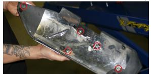
7. Install supplied cover mount bracket to side cover using OEM hardware.
