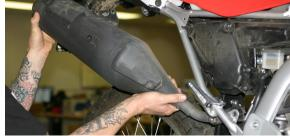
Install TBR slip tube and OEM mounting bolt.
