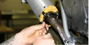
Remove side cover from heat shield. Save hardware for next step.
