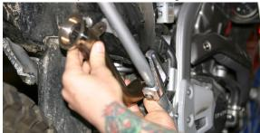
Install TBR muffler to TBR slip-on using the supplied 6x14mm socket head cap scews and lock washers provided. Leave loose for now. Use supplied 8x45mm socket head cap screw for upper muffler mount using the OEM washer and nut. Leave loose for now.
