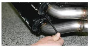
13. Tighten barrel clamp.
