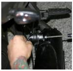
12. Tighten the 8 6x14mm socket head cap screws.
