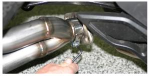
4. Before you run the bike, clean off all fingerprints and dirt, as any oily residue will etch the metal and become somewhat permanent when the system gets hot. Run the bike and enjoy. It is normal for some white smoke to appear the first time you start the bike. This is packing/manufacturing oil from inside the pipe burning off. Check for gaps or leaks. If you find a leak, a little high temperature silicon sealant should fix it. After 50 to 100 miles, recheck all fasteners for tightness.
