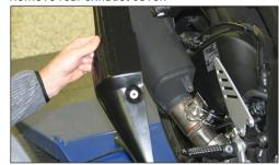
Remove exhaust valve cables from servo under seat. Use a wrench to hold server wheel in place or internal gears may break.
