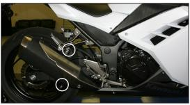
Remove clip and bolt from passenger foot peg, replace with 6x45mm bolt.
