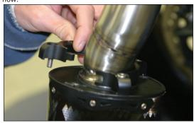
Install muffler assembly to motorcycle using the supplied barrel clamp and rubber lined muffler clamp, secure muffler to standard mounting position using OEM bolt and nut. keep loose for now.
