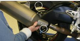
Install TBR muffler to slip-tube shown using the supplied 2-piece X-Ring and bolts with lock washers, keep loose for now.
