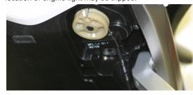
Remove the lower fairing bolt from left side of motorcycle to access o2 sensor and remove sensor.
