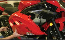
3. Remove the right foot rest assembly to access muffler mounting bolts.
