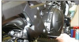
9. Slide the (rubber-lined) muffler clamp over the muffler canister and install header on bike using supplied flange bolt and nut on muffler clamp.
