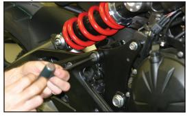
4. Remove muffler mounting hardware.
