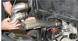
5. Remove 6 header flange bolts and remove OEM header system.
