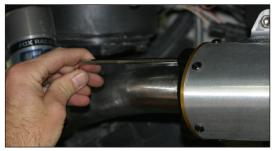
sides and secure in place with supplied 8x25mm bolts with lock nuts to mounting bracket.
