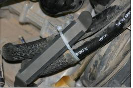
drivers seat. Loosely wrap hoses and bracket with supplied ziptie, make sure you have rubber side down on bracket.
