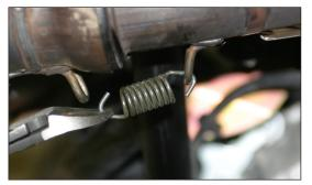
4. Remove exhaust pipe joint springs(2) above rear right wheel.
